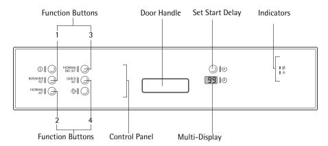
The **control panel** consists of the ON/OFF button ① and the programme buttons with LED displays.
